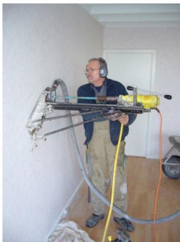
Figure 5.1: Drilling of concrete cores for testing
