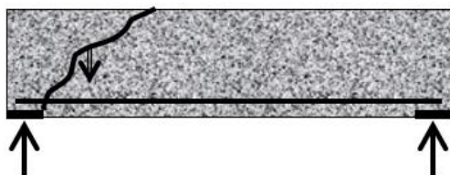
Figure 9.3: Failure mechanism in non-shear reinforced members
