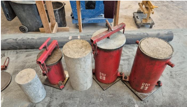
Figure 3.1: In-situ cast concrete specimens for compression testing
